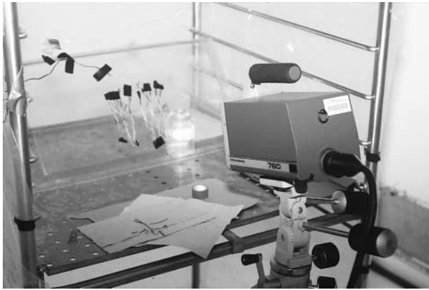
Fig. 1. Infrared thermal imaging radiometer and turfgrass plants in a controlled environment room.
